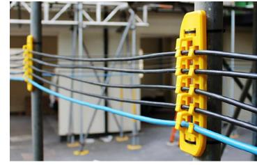
to keep the workplace in a safe operating condition. The open-ended design allows for quick, one-handed installation, while still providing up to a 340 pound load rating from the glass-filled polyester material. The CableSafe® safety hooks are multi-purpose and can be removed and re-used at another site.
