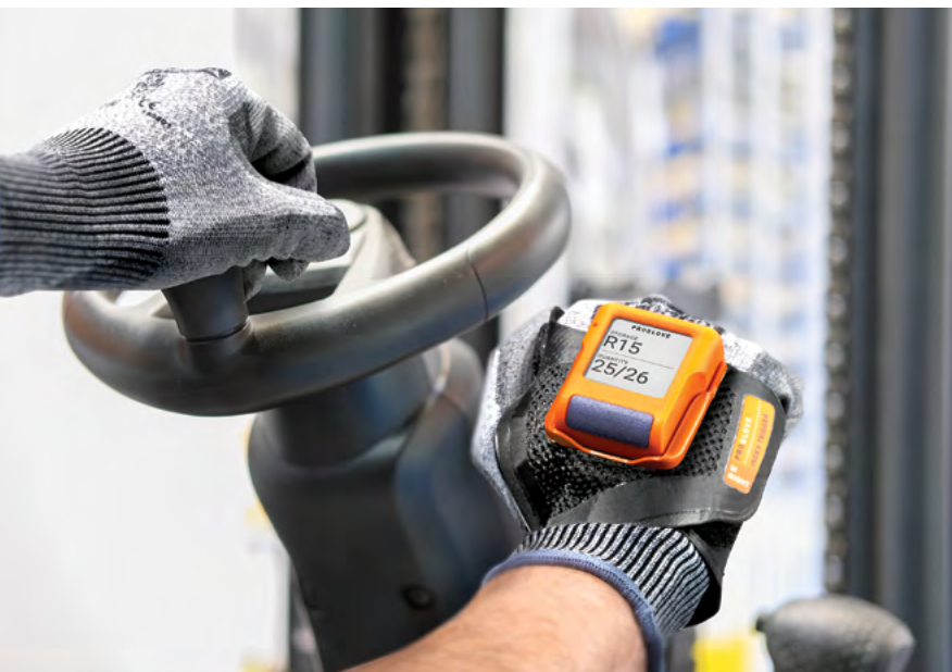
Tools like an ultralight wearable barcode scanner from ProGlove provide an ergonomic approach to hand protection and leave hands free for other tasks. (photo courtesy ProGlove)
