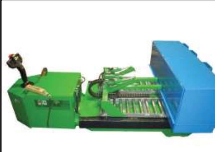
Die shown in cross-wise position preparing to install into press
