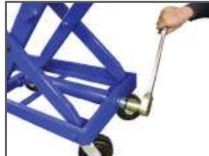
ACME screw operated units can be operated via air or electric impact wrench or manual ratchet
