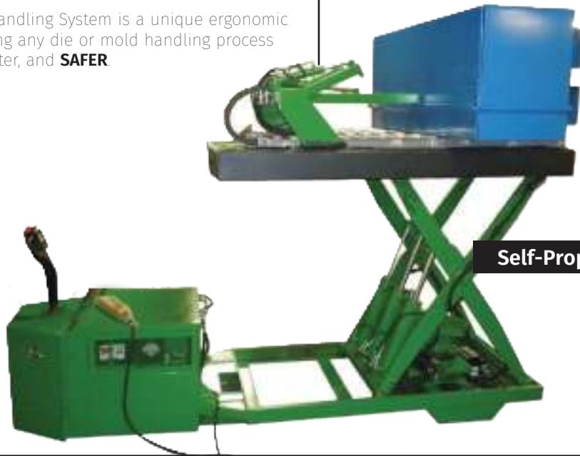
Die shown in cross-wise position preparing to install into press
