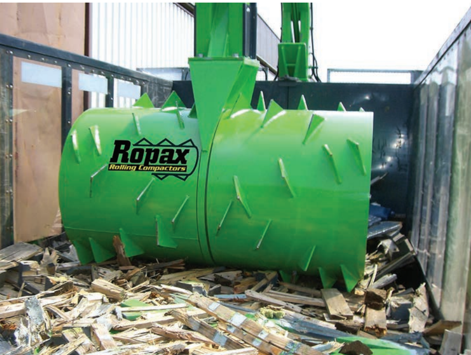
Rolling compactors consist of a two-ton steel roller drum at the end of an articulated boom. The surface of the drum is covered with sharp, spiked, teeth-like protrusions. There are many options available to help minimize waste-disposal costs. (photo courtesy Epax Systems, Inc.)
