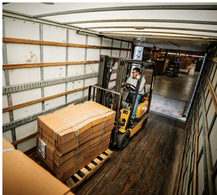
Keeping loads within the forklift's weight capacity reduces the risk of the forklift tipping over. Image courtesy of PERC.
