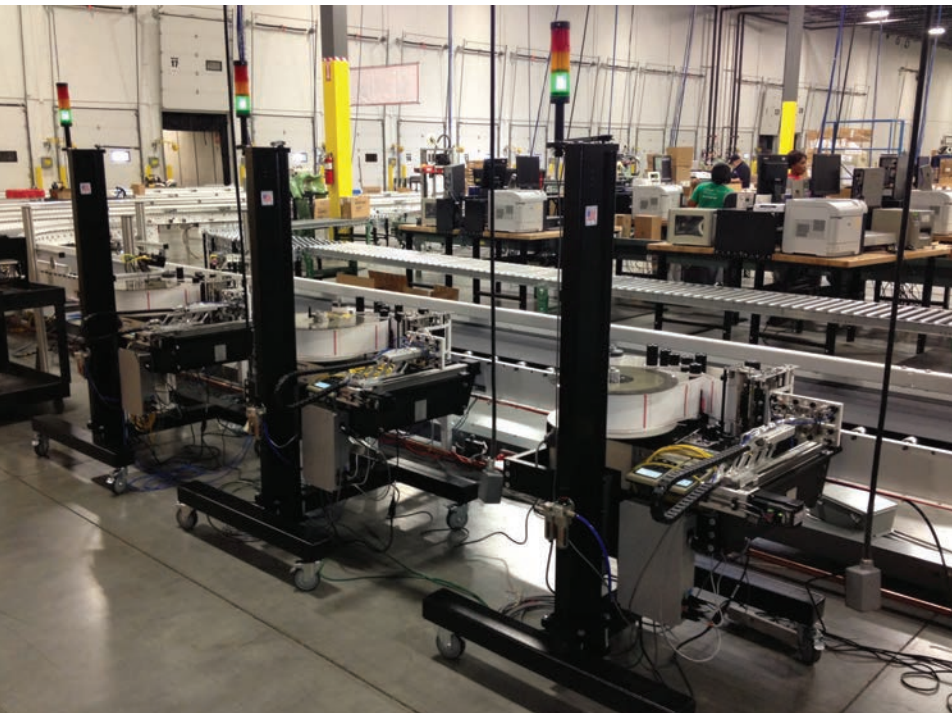
FOX IV Technologies has developed a product that automatically prints and applies shipping labels and the packing slip on one label. Image courtesy of Fox IV Technologies.
