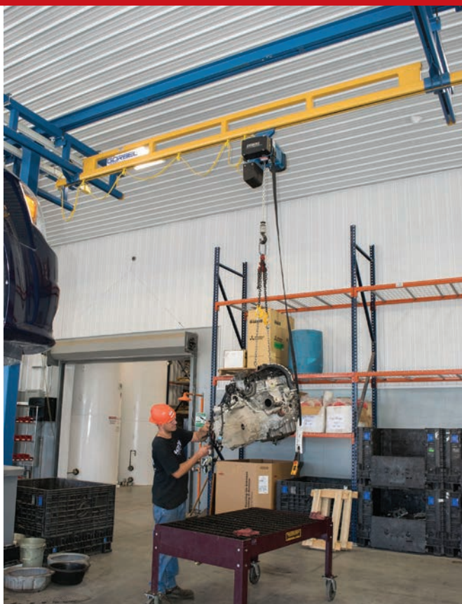
Pairing a workstation with an intelligent lifting device makes control more precise and enhances operator safety. Image courtesy of Gorbel.
