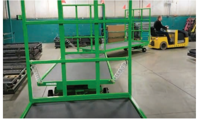
Tugger carts are connected by a towbar at front and a coupler at rear. Image courtesy of Topper Industrial.
