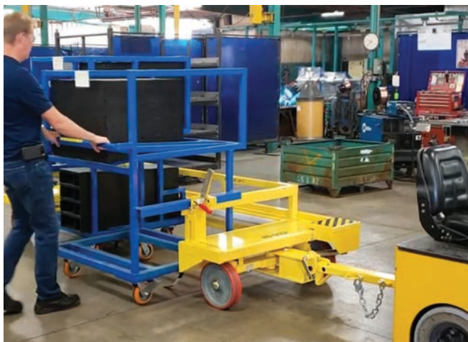
Daughter carts are pulled out and pushed back into the Mother Cart frame. Image courtesy of Topper Industrial.
