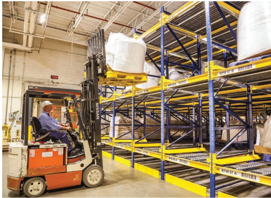
Racking inside distribution warehouses need to be protected with barriers to forklift traffic, such as guardrails.
