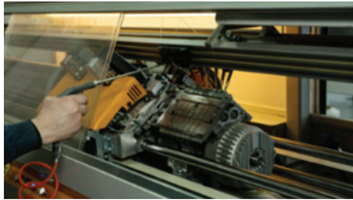
Smooth extruded aluminum and clear panel material act as a protective guard for this mechanized equipment.
