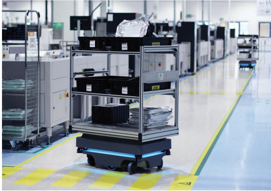
Visteon Electronics' fleet of four AMRs free employees from heavy, monotonous and low-value material-moving tasks. Photo courtesy of Mobile Industrial Robots
